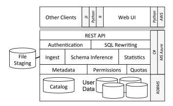
Figure 3: SQLShare architecture, primary user interface is the Web UI which communicates with the REST layer for dataset ingest, modification (via views) and querying. REST server interacts with the backend database which also keeps a catalog of user queries.
